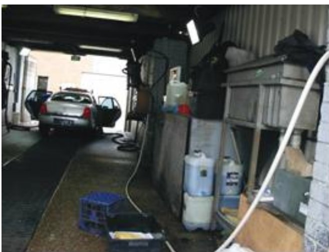
Figure-23: Recycling ( after separating oil from used water ) of treated water at car washing station in Sydney- Australia
