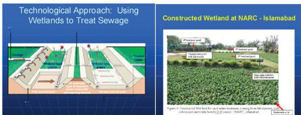
Figure-15: Schematic diagram / process flow and functional Hybrid constructed wetlands - NARC, Islamabad
