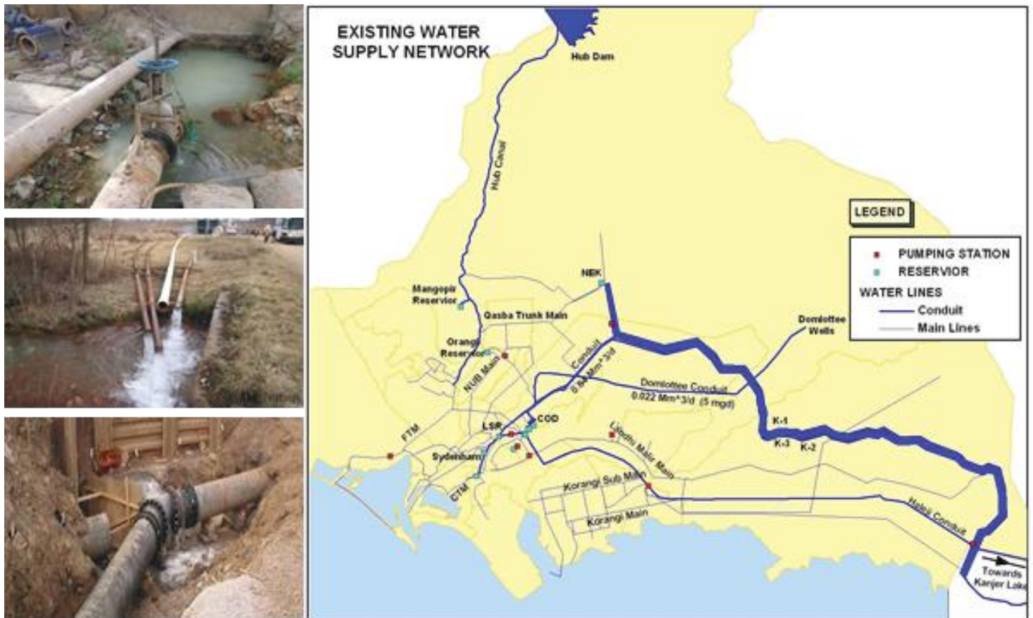
Figure-5: Existing water supply network and its present status ( leaking & outlived pipes ) - Karachi metropolitan
